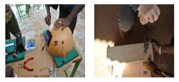
All sorts of materials are suitable for making a casing, including larger calabashes with a wooden board as bottom. Number and size of the holes depend on the parts to be fitted. A small drawing before drilling will be helpful. The drawing will show where the charge controller, the connectors and the switches are to be fitted.
