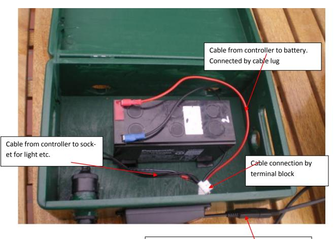
Cable from charge controller to solar module
