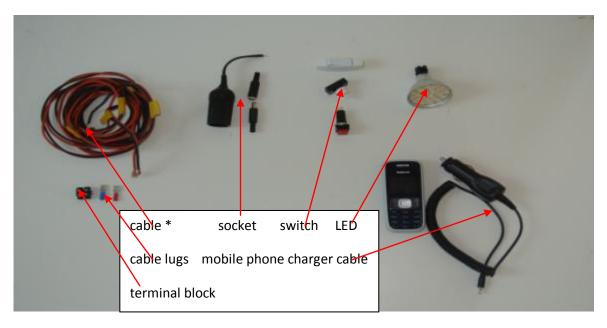
\* The cable connecting the solar module with the solar controller should be 2.5 mm thick and 5 m long; the cable to the light source should be 1 to 1.5 mm thick and 10 m long since the cables in West Africa are usually not made of copper but of an iron alloy. The stronger the cable, the better!
